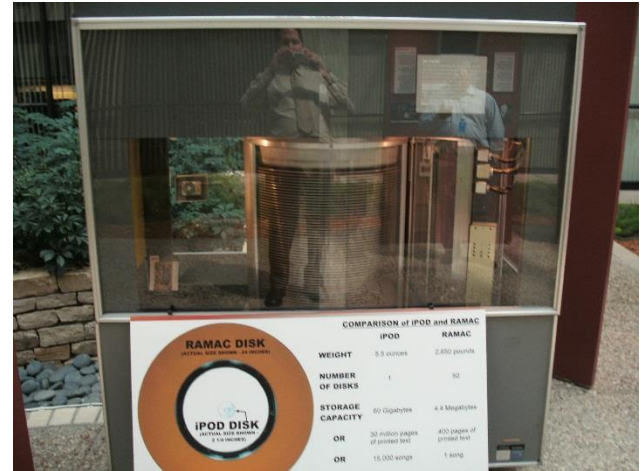
1956 IBM RAMAC disk drive 2650 lbs, cost $63,450 Stored 4.4 Megabytes
